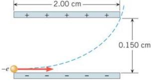
The electric field provides the force which creates an acceleration in the y direction. The acceleration in the y direction can act only for the time it takes the electron to travel 2.00 cm in the x direction.
