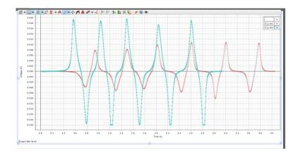
The horizontal axis is time in seconds, you could make use of this to find either speed or some other time related quantity. The vertical axis is voltage which is of course the EMF induced in the coils.
