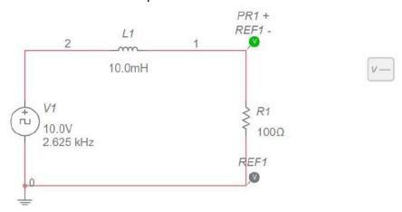
This time one measures the voltage across the resistor and one finds the equation is
