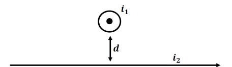
Two wires are shown above. Wire 1 carries a current  $i_1=15.0~\mathrm{A}$  straight out of the paper. The wire has a length of  $L_1=1.78~\text{m}$ . Wire 2 carries a current  $i_2=27.0~\text{A}$  going to the right. The wire has a length of  $L_2=4.92\ m$ . Wire 1 is located above wire 2 by a distance of  $d=0.39\ m$ . What is the magnitude of the magnetic force that Wire 1 exerts on Wire 2.
