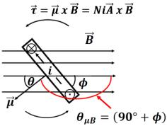
As shown above the right-hand rule puts the area down to the left. The cross product therefore results in a counter-clockwise rotation as shown. So, we see the coil will rotate counter-clockwise. The magnitude of the torque is
