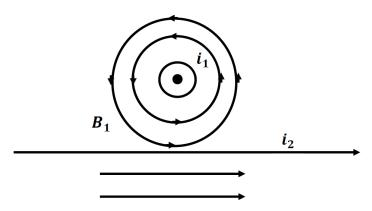
The B field for Wire 1 is concentric circles going counter-clockwise as shown above. The magnetic force of wire 1 on wire 2 is given by
