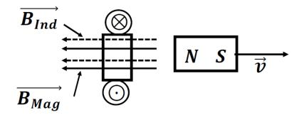
Because of the bar magnet, the magnetic field in the coil is initially pointing from the North pole or to the left. With the bar magnet, moving away from the coil, the field strength is decreasing. The magnetic flux is therefore decreasing. To oppose the change in magnetic flux, the induced magnetic field must go to the left to strengthen the decreasing magnetic flux. To create an induced magnetic field to the left, the current must go into the paper at the top of the coil!
