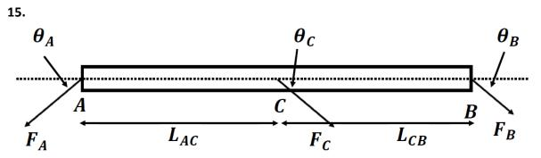
As shown above a massless board has three forces acting on it. The lengths are:  $L_{AC} = 2.34 \text{ m}$ , and  $L_{CB} = 2.34 \text{ m}$ . The forces are  $F_A = 12.7 \text{ N}$ ,  $F_B = 21.3 \text{ N}$ , and  $F_C = 18.6 \text{ N}$ . The angles are  $\theta_A = 34.5^\circ$ ,  $\theta_B = 28.9^\circ$ , and  $\theta_C = 41.1^\circ$  Determine the magnitude and direction of the net torque about
