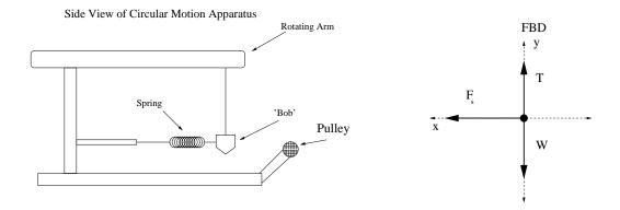
From the FBD for this system, we see that the circular motion of the 'Bob' is caused by the force supplied by the spring,  $F_s$ . This force is constant throughout the experiment. The net force in the x-direction is thus the spring force. This then is equal to the centripetal force so we can represent this as
