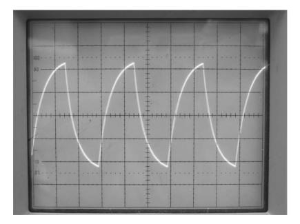
This is known as a shark tooth signal. The capacitor is just reaching full charge for a moment and then it is discharging. If you have a shorter height and you have a sharp point at the top, then you are not fulling charging the capacitor and your frequency is too high, try lowering it some.
