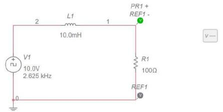
This time one measures the voltage across the resistor and one finds the equation is
