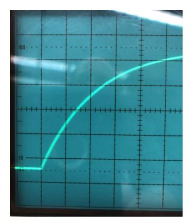
Notice how the curve comes to touch the 0% line and a vertical line that we can now use as a reference to mark the start of time. If the curve does not go all the way down such as this picture shows
