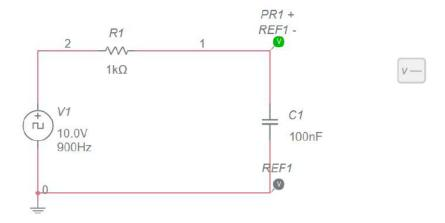
Consider the following circuit composed of a resistor and a capacitor
