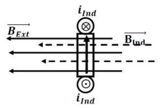
The external magnetic field due to bar magnet has the field pointing to the left. Since the magnet is moving away from the coil, the strength of the magnetic field is decreasing. Therefore, the magnetic flux through the coil is decreasing. So, the induced magnetic field must also go to the left to strengthen the field and oppose the decrease in flux. Therefore, by the right-hand rule, the current must be induced going into the paper at the top and coming out of the paper at the bottom.
