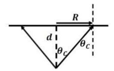
The critical angle where the refracted ray going from water to air is  $90^\circ$  can be found from Snell's law
