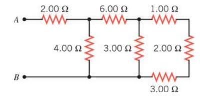
Always start away from where you are trying to find the resistance between. So we begin by combining the 1 $\Omega$ , 2 $\Omega$ , and 3 $\Omega$  in series.
